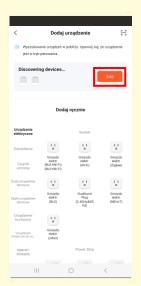
3.On the interface ,you will find "Devices to be added",choose go to add.For no response,4 short and 1 long press on motor PROG button to reset
